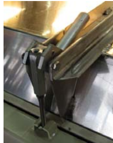
Fast and Easy Screen changes with our Quick-Release Clamps.
